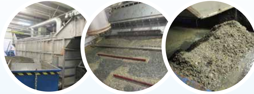
Sedimentation tank Floating particle separation Heavy particle collection
