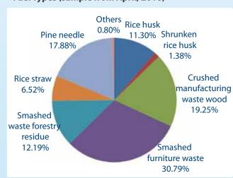
The plant was designed for rice crop residues, but the quality and flexibility of the technology has enabled the use of other waste products.
